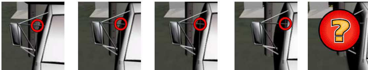
Antenna and mirror support bar create a feature which does not correlate to a real-world feature
