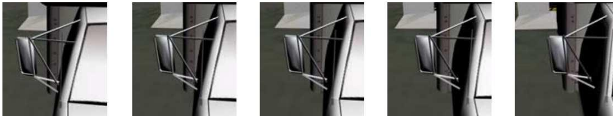
Antenna and mirror support bar create a feature which does not correlate to a real-world feature
